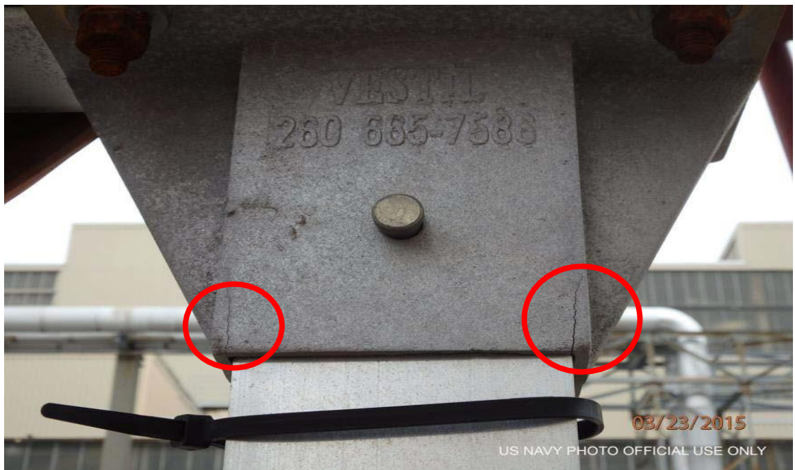
Cracks in Cast Upper Mounting Brackets
